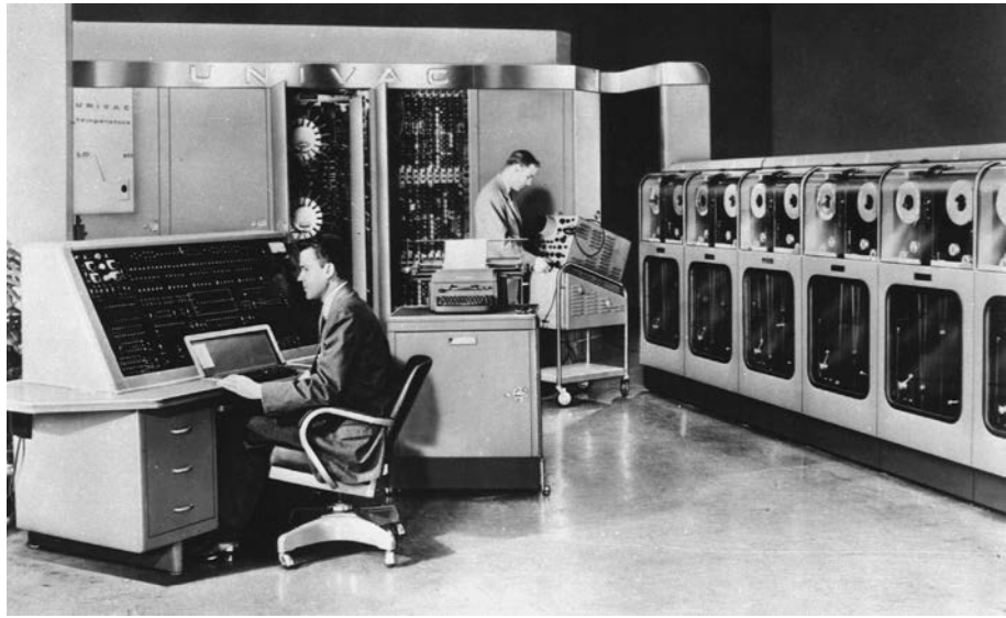
FIGURE e1.13.2 UNIVAC I, the first commercial computer in the United States. It correctly predicted the outcome of the 1952 presidential election, but its initial forecast was withheld from broadcast because experts doubted the use of such early results.
