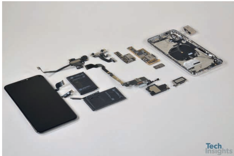
FIGURE 1.7 Components of the Apple iPhone Xs Max cell phone. At the left is the capacitive multitouch screen and LCD display. Next to it is the battery. To the far right is the metal frame that attaches the LCD to the back of the iPhone. The small components surrounding in the center are what we think of as the computer; they are not simple rectangles to fit compactly inside the case next to the battery. Figure 1.8 shows a close-up of the board to the left of the metal case, which is the logic printed circuit board that contains the processor and the memory (Courtesy TechInsights, www.techinsights.com ).
