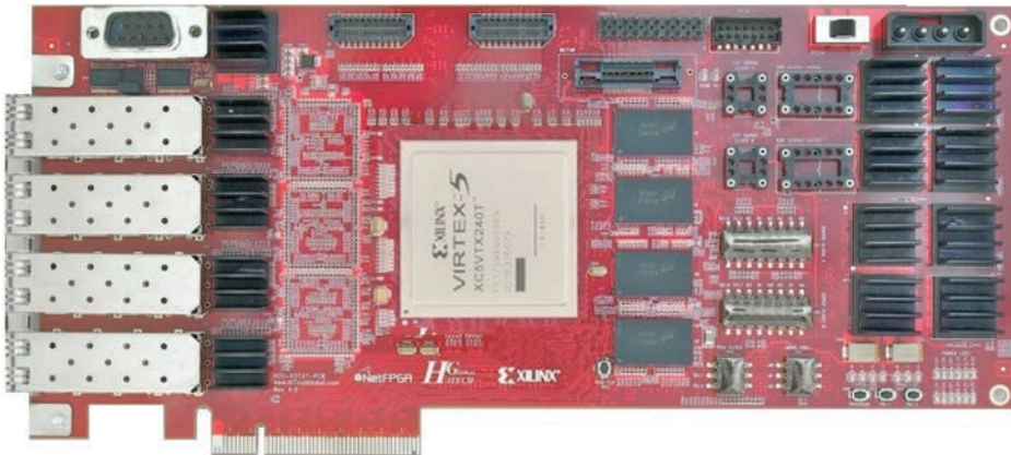
FIGURE e6.10.1 The NetFPGA 10-Gigabit Ethernet card (see http://netfpga.org/ ), which connects up to four 10-Gigabit/sec Ethernet links. It is an FPGA-based open platform for network research and classroom experimentation. The DMA engine and the four “MAC chips” in Figure e6.10.2 are just portions of the Xilinx Virtex FPGA in the middle of the board. The four PHY chips in Figure e6.10.2 are the four black squares just to the right of the four white rectangles on the left edge of the board, which is where the Ethernet cables are plugged in.
